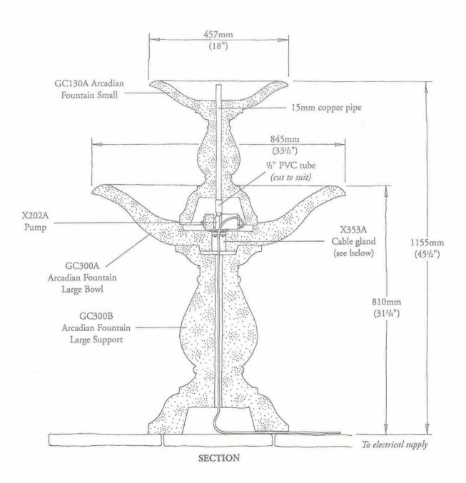
Cable Gland - Remove brass plug and pass electrical cable through gland. Top plates must be attached to bottom plates at  $90^{\circ}$  to achieve seal. Tighten bolts using 4mm allen key/hex wrench.
