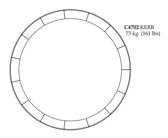
$\emptyset$  10mm  $\binom{3}{8}$ ") stainless steel dowels (not supplied) 50mm (2") projection into stone. Holes to be drilled on site to suit by others. Minimum of 2 No dowels per stone secured using a flexible building adhesive such as Evode Serious Stuff, Loctite Fast Grab, or similar
