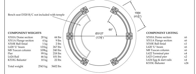
Read in conjunction with Tech Sheet T11, T14, T35 and CAD1 All weights are approximate and should be used as a guideline only All dimensions exclude joints - allow 6mm  $\binom{1}{4}$  for vertical and bedding joints
